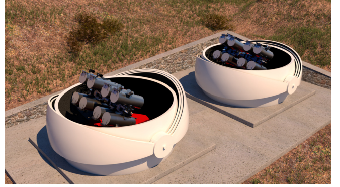
Figure 16. Visualisation of a full GOTO node site consisting of 16 UTs spread over 2 domes. The northern and southern nodes will contain identical sets of 2x8, providing a total of 32 UTs.
